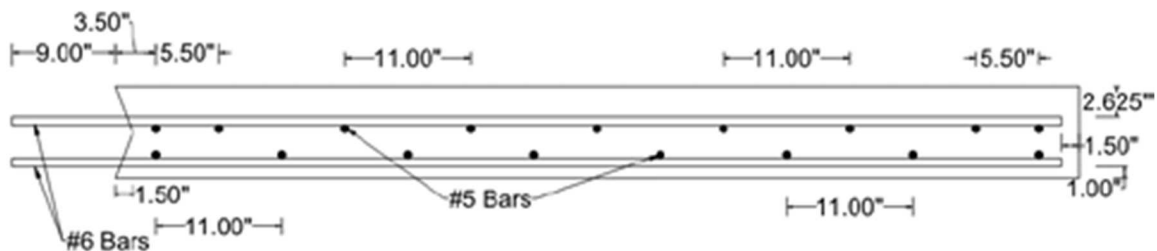
Figure 3-5. Cross Section of Left Deck Panel
