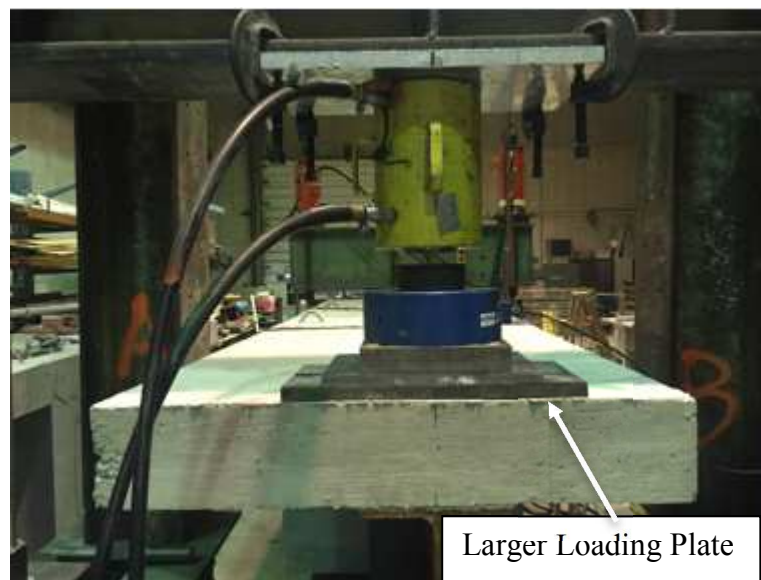
Figure 4-24. Revised Loading Configuration of Specimen I
